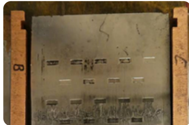
Fig. 8: Meniscus of moulds after 1500 heats
